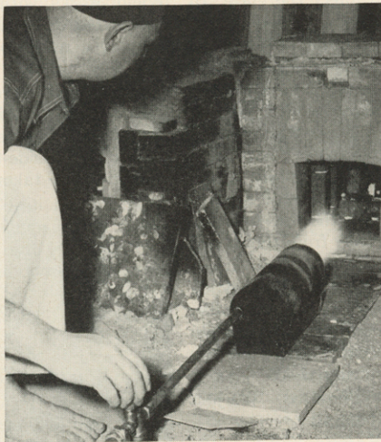
Kjeld heats his kilns with this burner which looks like a large blowtorch, moving it nearer as the firing advances. Kerosene is the fuel
